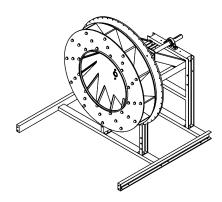
2. Fit rear panel to support. Slide impeller on drive shaft.
