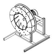
2. Fit rear panel to support. Slide impeller onto shaft.
