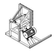
Screw individual parts of fan support together.
