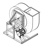
3. Screw housing to fan rear panel.
