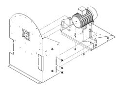
2. Bolt motor bracket together and attach motor
