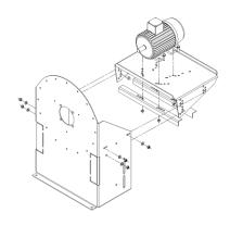
1. Bolt motor bracket together and attach motor
