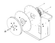
2. Mount back plate and impeller
