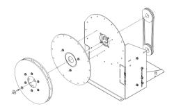
3. Install V-belt drive. Tension drive belts. Mount back plate and impeller
