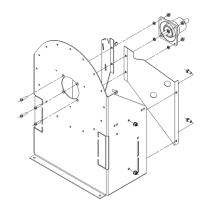
1. Install flanged bearings and reinforcement plates
