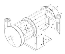
4. Install casing and V-belt protection
