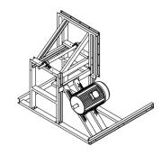
1. Screw individual parts of fan support together. Fit bearing units and shaft on support. Fix motor to support.
