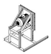
1. Screw individual parts of fan support together. Fit motor on support.
