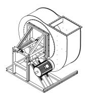
3. Screw housing to fan rear panel.
